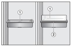
It consists of a deep tray ① and a shallow tray ②. Both trays fit the stainless steel frame.
